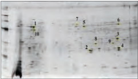
Figure 38. 2D gel stained with the Pierce Silver Stain for Mass Spectrometry. Proteins of a rat mitochondrial extract were separated by IEF (pH 5–8 gradient) and SDS-PAGE, then stained. Ten spots were identified that stained well in three identical gels that were stained with three different stains (Table 30). These spots were picked for in-gel digestion and MS analysis.
